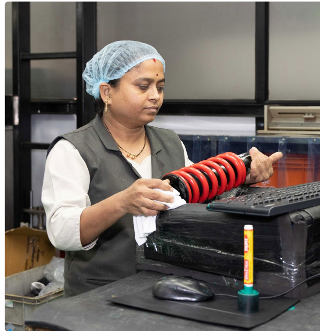
Final inspection of mono-shock assembly, Chh Sambhajinagar
