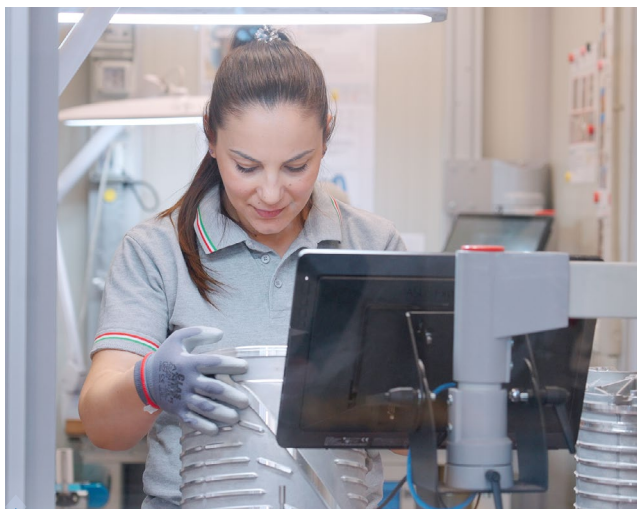
Visual control on stator housing at Endurance SpA plant, Italy.
