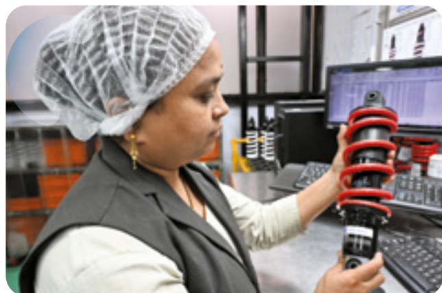
Final inspection of rear mono-shock absorber
