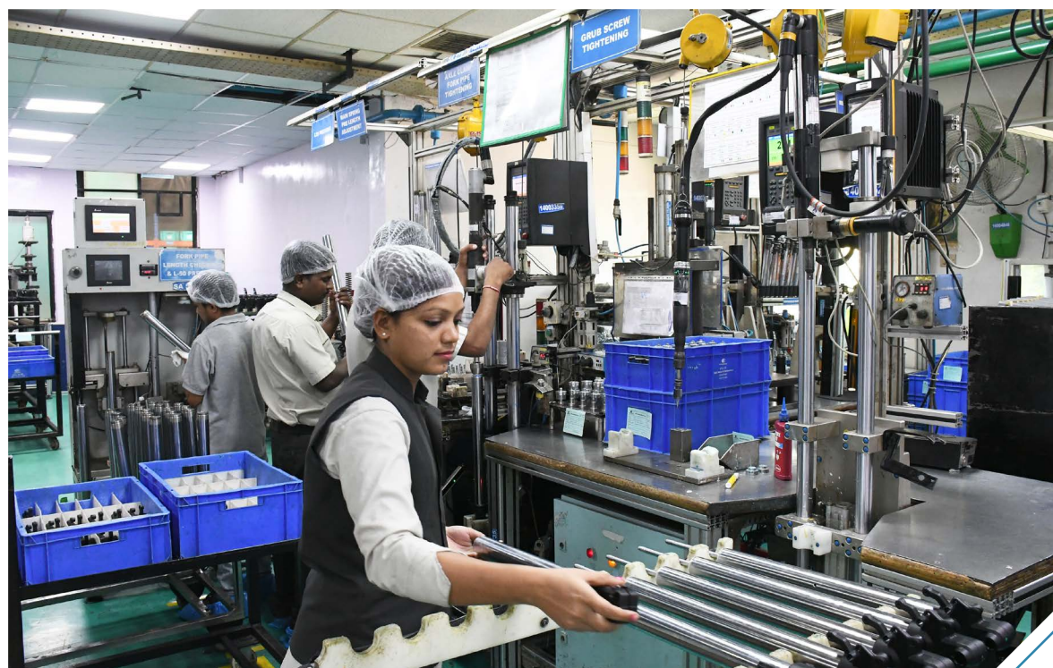
Inverted Front Fork Assembly Line Suspension Plant at E-93 Waluj, Aurangabad
