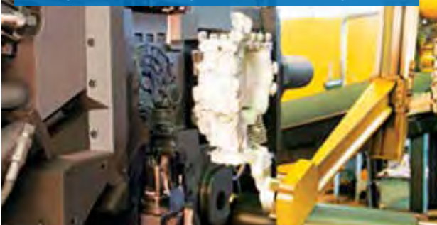
Casting - 1,350 tonne High Pressure Die Casting Machine
