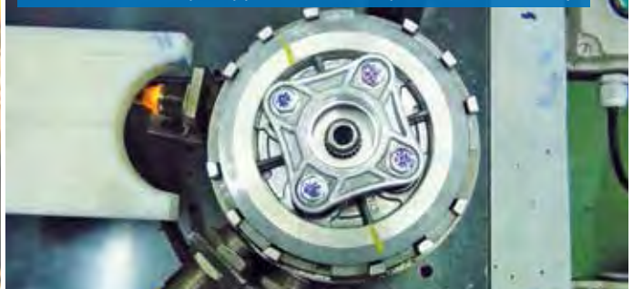
Transmission - Torque application on wet-plate clutch assembly
