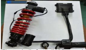
Electronically Controlled Suspension (Fully developed In-house)
