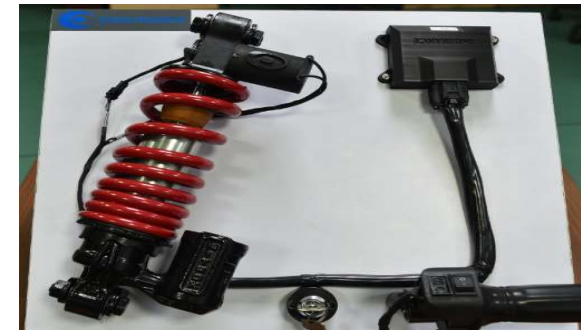
Electronically Controlled Suspension (Fully developed In-house)
