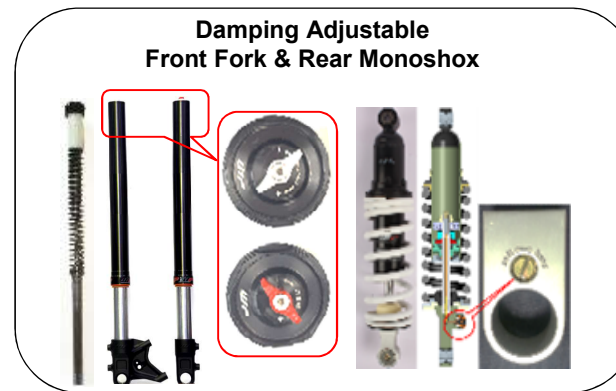
Electronically Controlled Suspension (Fully developed In-house)
